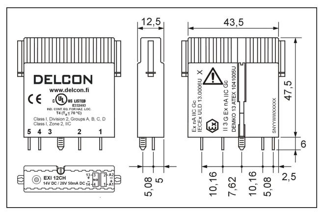
EXI 12CH (dimensions in mm, nominal). Markings can be located differently by production lot. Production lot number is marked to the relay (SN = serial number YY = year, WW = week, XXXXX = lot number).
