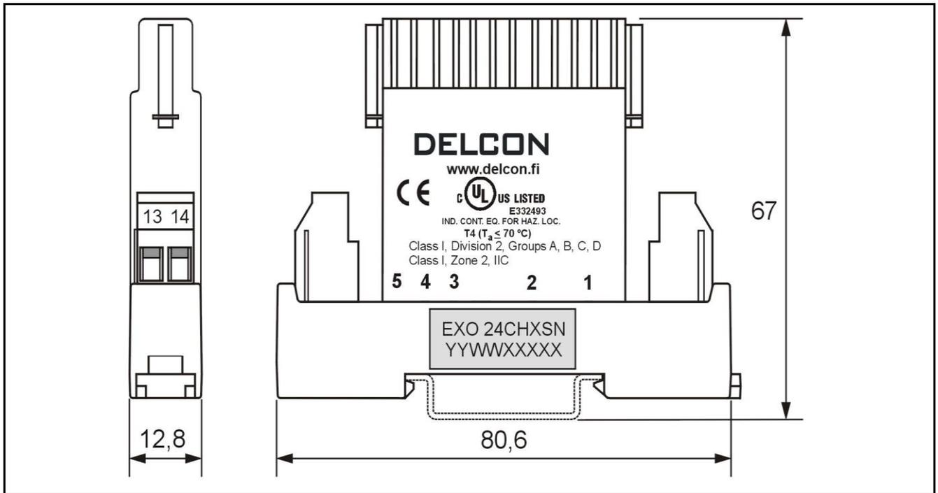
EXO 24CHXSN (dimensions in mm, nominal). Markings can be located differently by production lot. Parts of the markings are backside of the relay. Production lot number is marked to the socket (YY = year, WW = week, XXXXX = lot number).
